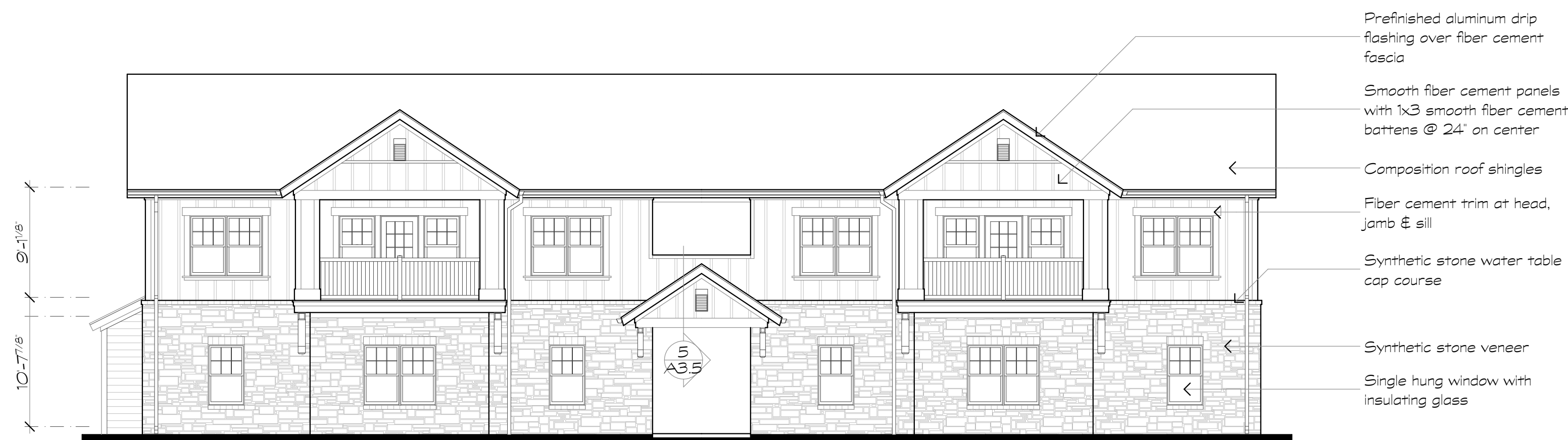
2 Building Type IV Scale: 1/8" = 1'-0" Rear Elevation
