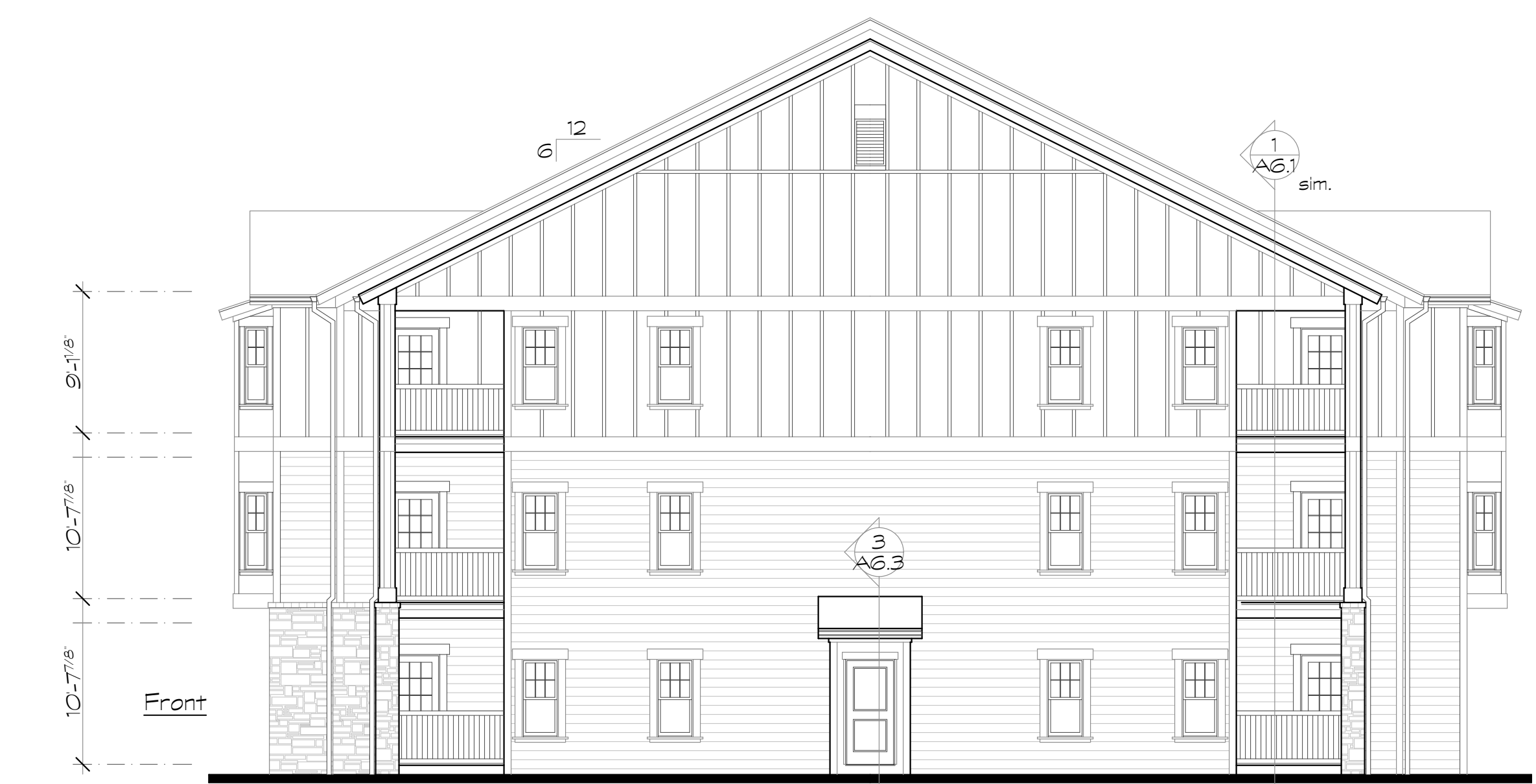
4 Building Type II - Bldg. 15 Scale: 1/8" = 1'-0" End Elevation
