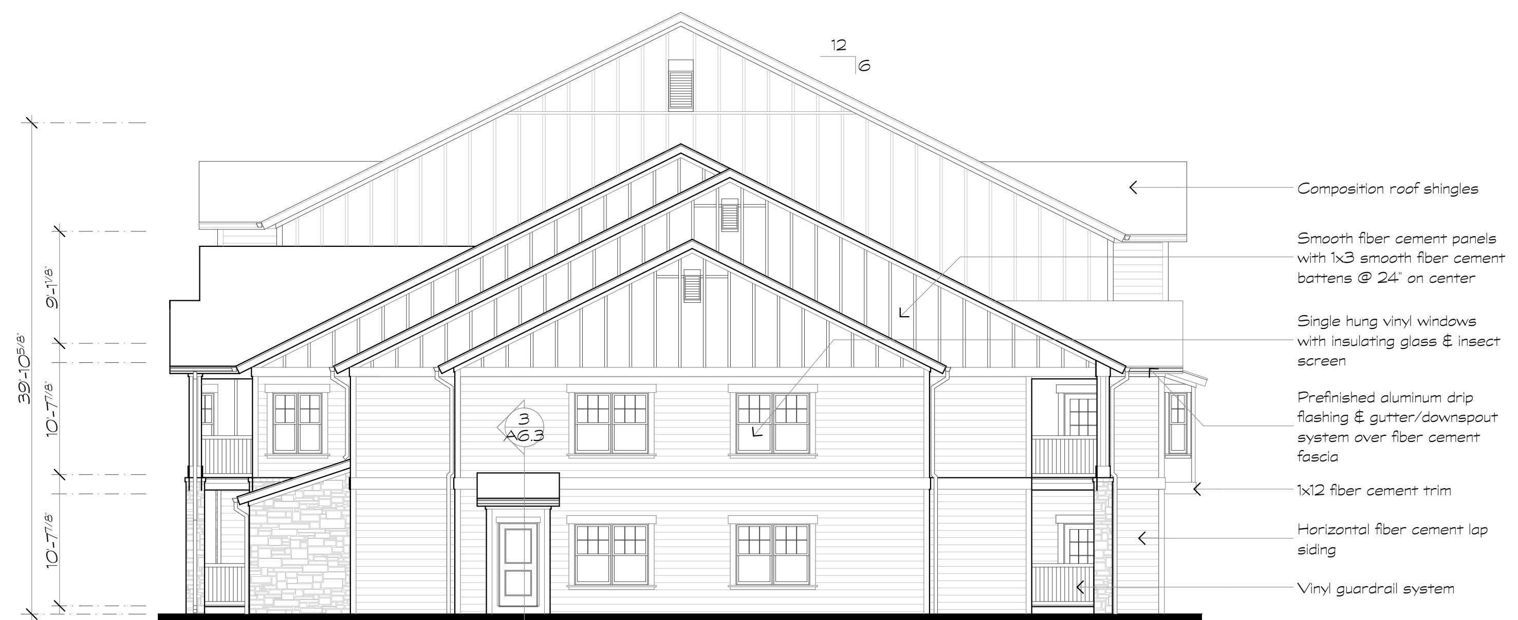
4 Building Type III - Bldg. 4 Scale: 1/8" = 1'-0" End Elevation
