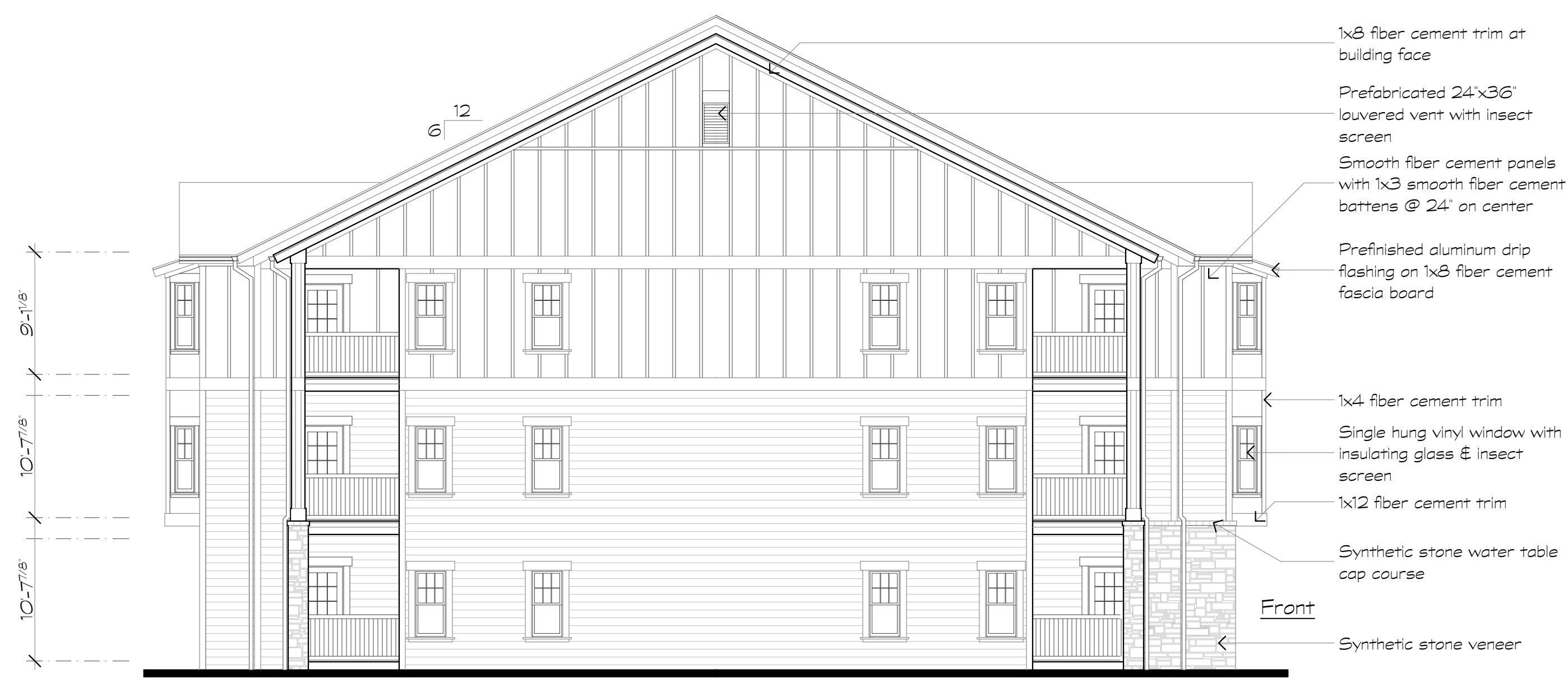
3 Building Type II - Bldg. 15 Scale: 1/8" = 1'-0" End Elevation
