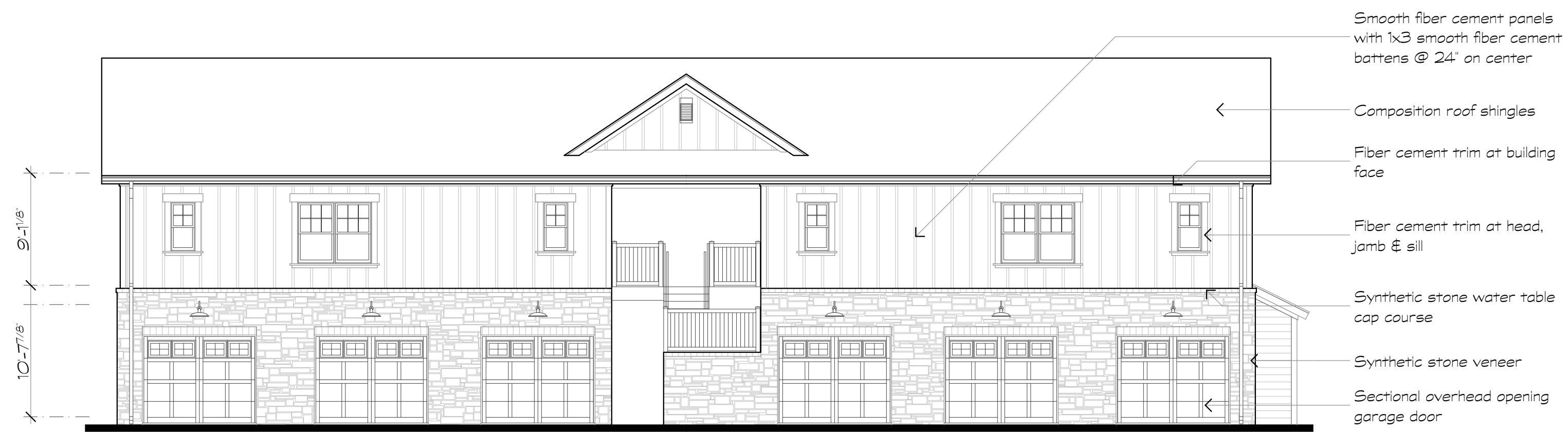
1 Building Type IV Scale: 1/8" = 1'-0" Front Elevation
