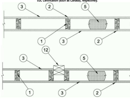
1. Wood Studs — Nom 2 by 4 in. spaced 16 in. OC max, effectively firestopped.
