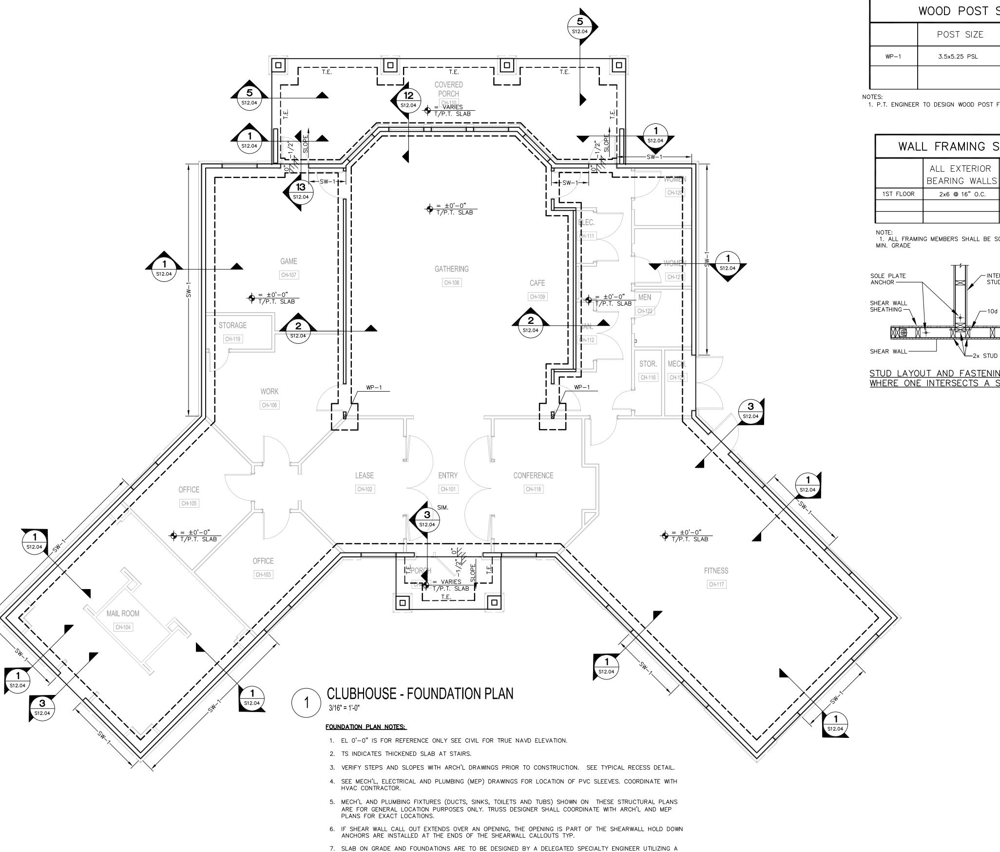
MINIMUM OF 4" CONC SLAB-ON-GRADE ON 10 MIL VAPOR BARRIER ON COMPACTED, TREATED SUB-SOIL (TYPICAL). EXTERIOR FOUNDATION EDGES SHALL BE MINIMUM 12" WIDE, AND CHAMPHORED BACK TO SLAB WITH
