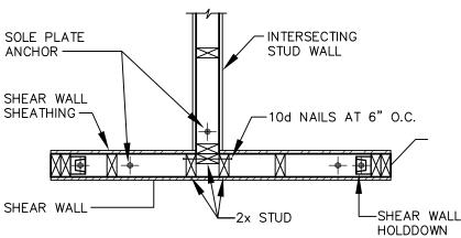
STUD LAYOUT AND FASTENING AT LOCATION WHERE ONE INTERSECTS A SHEAR WALL
