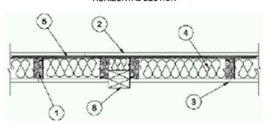
1. Wood Studs — Nom 2 by 4 in. spaced 16 in. OC with two 2 by 4 in. top and one 2 by 4 in. bottom plates. Studs laterally-braced by wood structural panel sheathing (Item 5). When Mineral and Fiber Boards\* (Item 5A) are considered as bracing for the studs, the load is restricted to 76% of allowable axial load. Walls effectively
