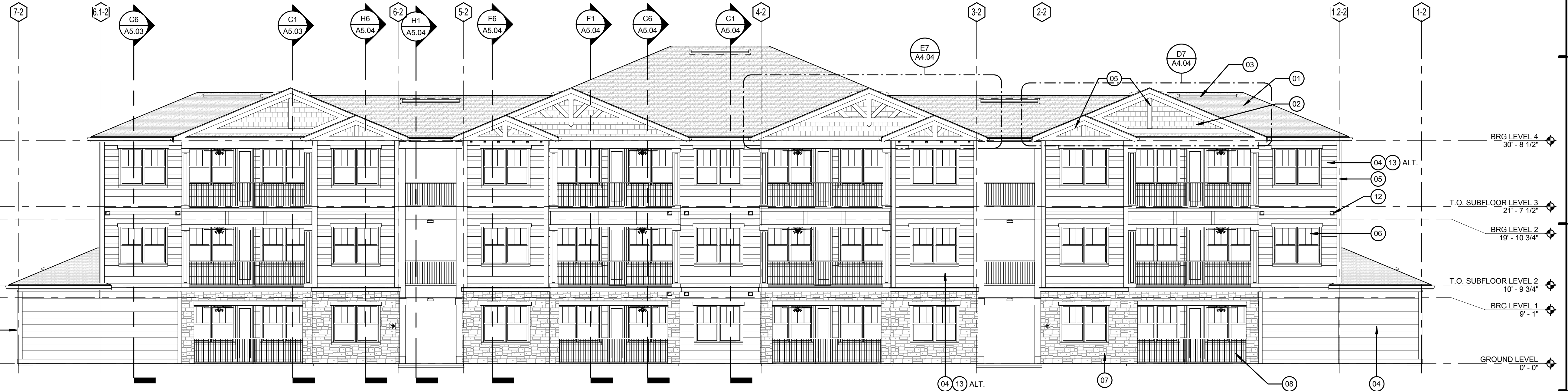
F1 BUILDING TYPE 2 - REAR ELEVATION 1/8" = 1'-0"
