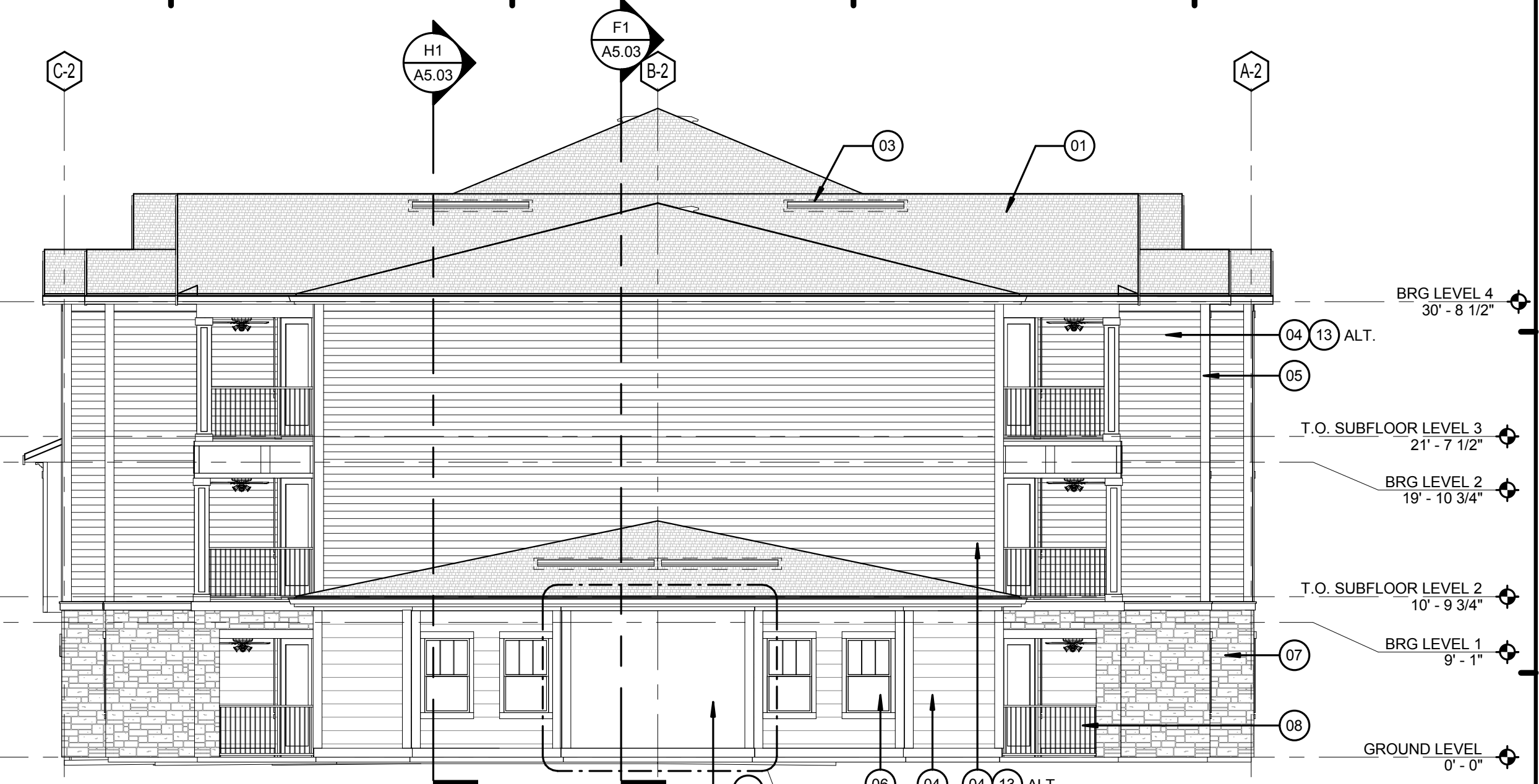
C6 BUILDING TYPE 2 - RIGHT SIDE ELEVATION 1/8" = 1'-0"
