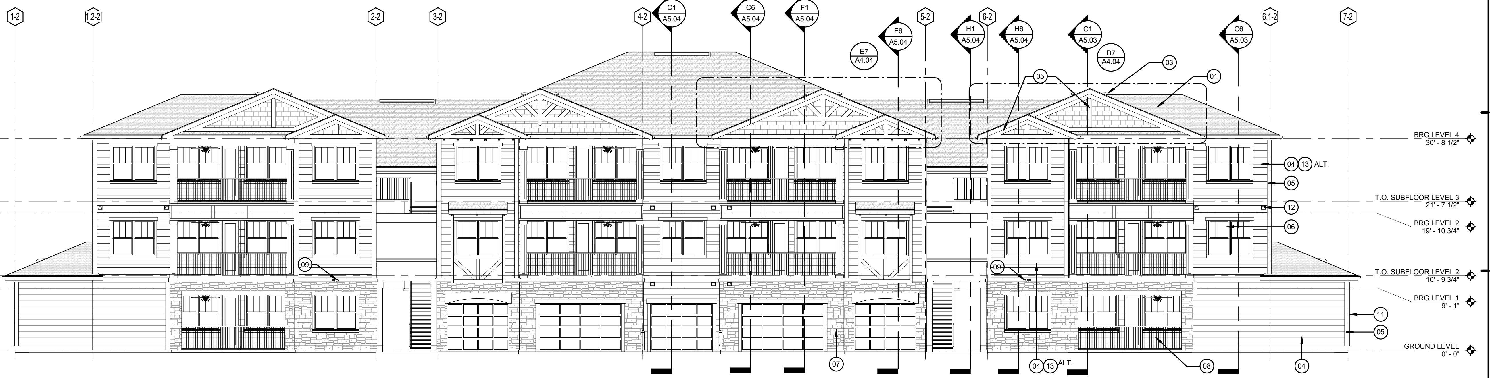
H1 BUILDING TYPE 2 - FRONT ELEVATION 1/8" = 1'-0"
